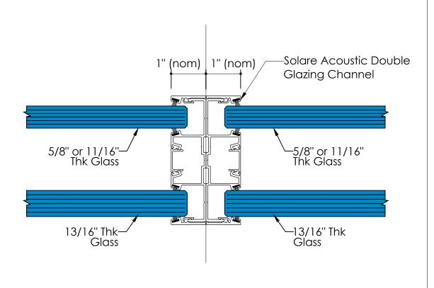
Solare™ Acoustic Double Glazed Partition System New Avanti DG Track to increased STC rating
