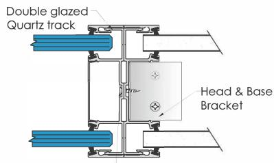
Quartz track screwed back to back as shown, to create mullion between head and base tracks.
