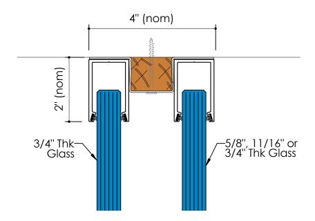
Solare<sup>™</sup> Acoustic Double Glazed Partition System Deep Deflection Track - Head
