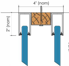
Asymmetric Glass Note: Tracks are factory manufactured to suit site glass specification.
