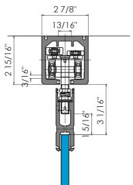
Movare™ Movable Single Glazed Partition System Characteristics Head Track: Center or End Fold Glazing Panel Width: 9 3/4" min. - 36" max.
