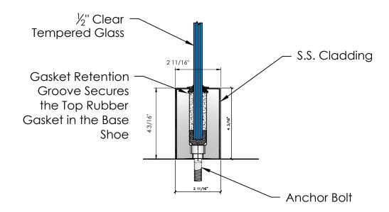
Solare™ Acoustic Single Glazed Partition System Characteristics Maximum Glazing Panel Width: 60" max. (custom widths available upon request) Maximum Glazing Panel Height: Full height up to 12 feet
