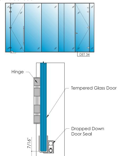
Solare™ Acoustic Single Glazed Partition System Characteristics Maximum Glazing Panel Width: 60" max. (custom widths available upon request) Maximum Glazing Panel Height: Full height up to 12 feet
