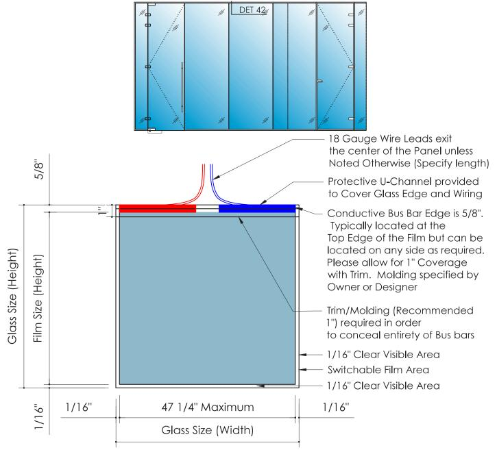
Solare<sup>™</sup> Acoustic Single Glazed Partition System Lunar<sup>™</sup> Smart Glass Characteristics Each switchable glass panel is controlled separately by single/ 3 way switches Maximum Glazing Panel Height: Full height up to 12 feet Maximum Glazing Panel Width: 4 feet
