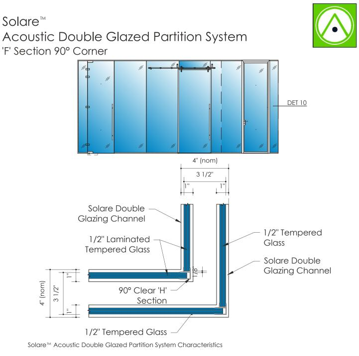
Maximum Glazing Panel Width: 60" max. (custom widths available upon request) Maximum Glazing Panel Height: Full height up to 12 feet Glazing Available: 3/8" Clear tempered, 7/16" Clear laminated, 1/2" Clear tempered, 9/16" Clear
