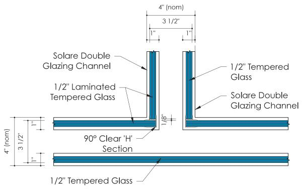
Solare™ Acoustic Double Glazed Partition System Characteristics
