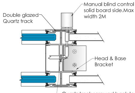
Quartz track screwed back to back as shown, to create mullion between head and base tracks.
