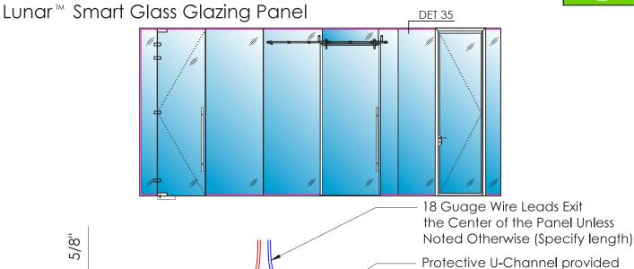
to Cover Glass Edge and Wiring Conductive bus Bar Edge is 5/8". Typically Located at the Top Edge of the Film But Can be Located on Any Side as Required. Film Size (Height) Please Allow for 1" Coverage with Trim. Molding Specified my Owner or Designer Trim/Molding (Recommended 1") Required in Ordered
