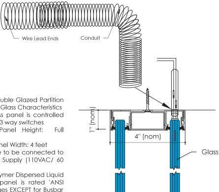
Solare™ Acoustic Double Glazed Partition System Lunar™ Smart Glass Characteristics Each switchable glass panel is controlled separately by single/ 3 way switches
