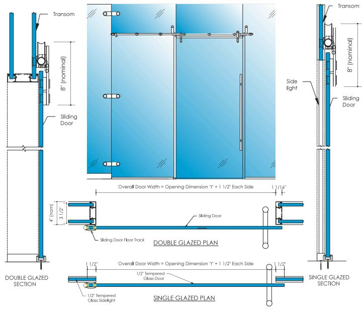
The Barn Sliding Glass Doors can be integrated with our interior glass partitions or with a standard wall to add a touch of modern style. Handles can lock into the floor, ceiling or both.
