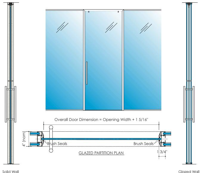
The Pocket Sliding Glass Door slides smoothly into any of our double glazed wall systems. It retracts between the fixed panels for an ultra-modern entryway.
