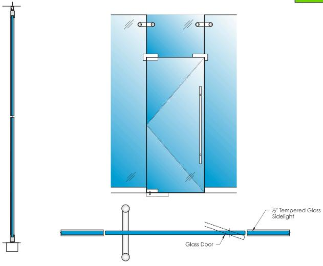
Pivot Frameless Glass Swing Doors are completely customizable. The two-way pivoting doors can fit with almost every system we offer and are available with numerous handle options with both locking and standard.
